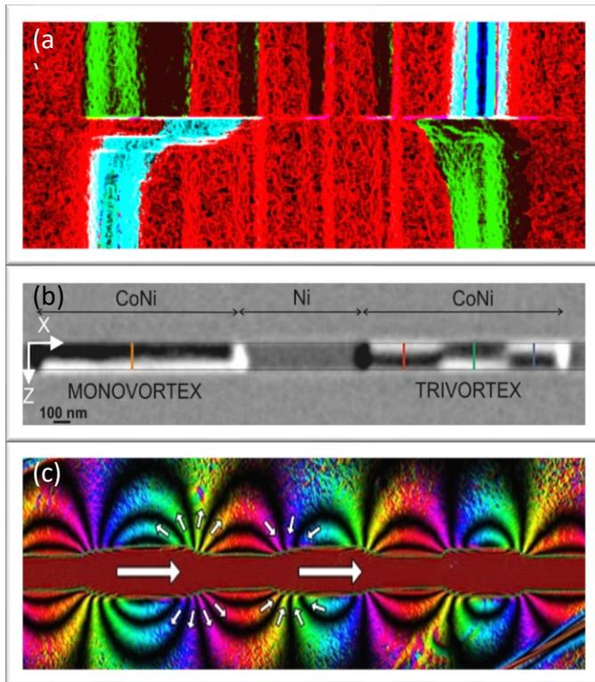
Figure: (a) Non-standard MFM image of a FeCo/Cu NW, (b) TXM contrast of a selected part of CoNi/Ni NW (c) magnetic flux image reconstructed from the magnetic phase shift images corresponding to a FeCoCu modulated NW.
